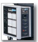
Nema 4 fiberglass enclosure makes a water-tight Control Box featuring conveniently positioned Hour Meter, Operational Indicator Lights. manual reset high temperature Cutout Switch, and Other Switches for exhaust fan, burner, auto fill pump, and foam suppression system. The side panel includes Troubleshooting Indicator **Lights** and a **Batch** Counter, which monitors the wastewater concentration level and automatically shuts down the system when
