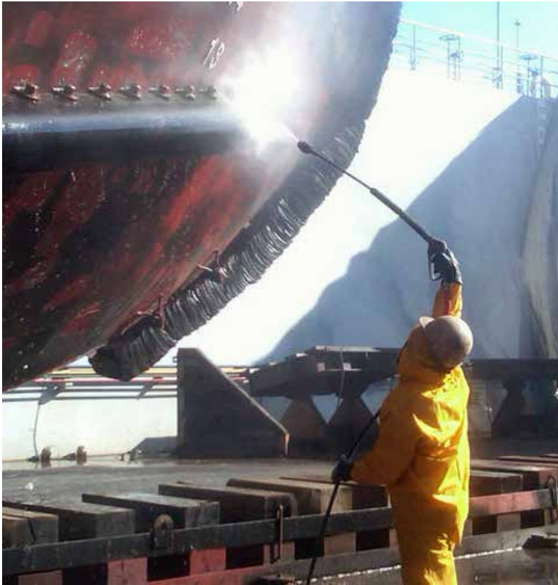
Cleaning a ship's hull is only one of the many applications for the MPE high-pressure washers with cleaning power of 5.0 GPM and 5000 PSI.
